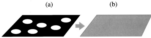
FIG. 1. Schematic representation of the homogenization procedure. The original heterogeneous boundary condition on the surface (a) is replaced by the homogenized partially absorbing boundary condition (b) characterized by the uniform trapping rate \kappa . On the heterogeneous surface, the boundary condition is D\nabla_n G(\mathbf{r}, t | \mathbf{r}_0) = \kappa_{disk} G(\mathbf{r}, t | \mathbf{r}_0) on the trap surfaces and \nabla_n G(\mathbf{r}, t | \mathbf{r}_0) = 0 otherwise, where G(\mathbf{r}, t | \mathbf{r}_0) is the particle propagator and \mathbf{n} is the surface normal vector. The boundary condition over the entire homogenized surface is given by D\nabla_n G(\mathbf{r}, t | \mathbf{r}_0) = \kappa G(\mathbf{r}, t | \mathbf{r}_0) .
